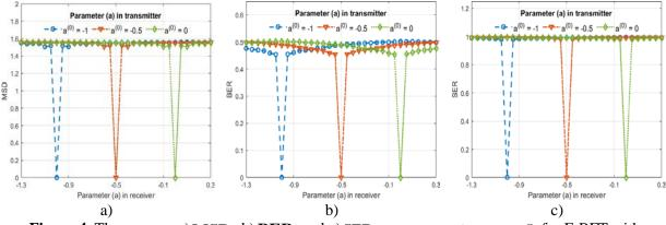
**Figure 4.** The average a) **MSD**, b) **BER** and c) **SER** measurements versus *a* for FrBFT with different values of parameter  $a^0$ :  $a^0 = -1$  (blue dashed circles),  $a^0 = -0.5$  (red dash-dotted triangles),  $a^0 = 0$  (green dotted diamonds). When parameters in transmitter (Alice) and receiver (Eva) are the
